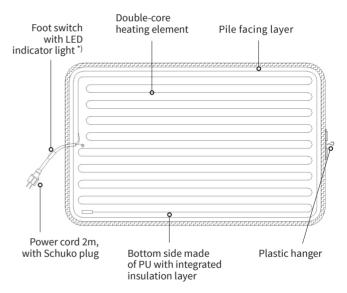
\*) The LED integrated in the foot switch indicates the operating status of the "Heated Carpet". If the LED lights up blue, the "Heated Carpet" is switched on. If the LED does not lit, the carpet is switched off.
